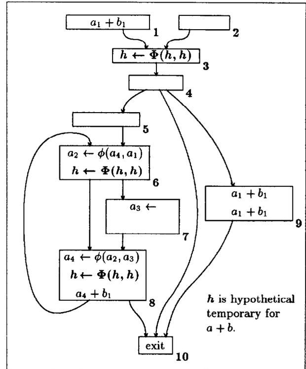
Figure 3: Program after  $\Phi$ -Insertion
